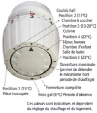
A thermostatic valve automatically maintains the temperature of a room. In fact, inside the rotary knob is hidden a mechanism that expands or contracts depending on the ambient temperature - and suddenly it opens or closes the hot water supply to the radiator.
